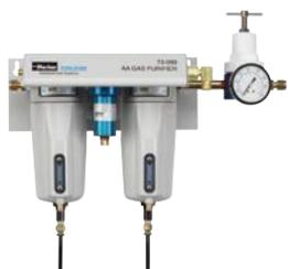
The 2-stage air filtration assembly consists of a Balston Grade DX coalescing filter and a Balston Grade BX coalescing filter. Together these filters remove oil, water and particulate contamination (99.99% at 0.01 micron) from the compressed air supply.
