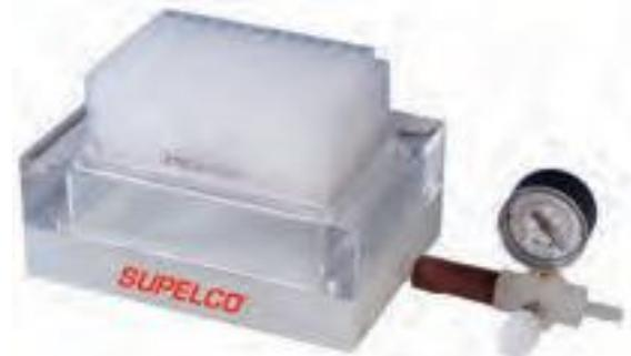
**Note:** The PlatePrep Vacuum Manifold is not compatible with the Empore 96-well plate
